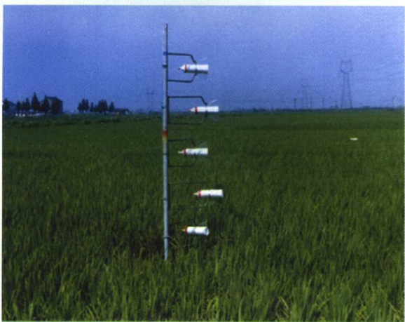
常熟农业生态站（江苏）水稻土氮挥发的微气象学测定 Microclimate measurement for estimating \text{NH}_3 volatilization from paddy soils, Changshu Experiment Station, Jiangsu Province
