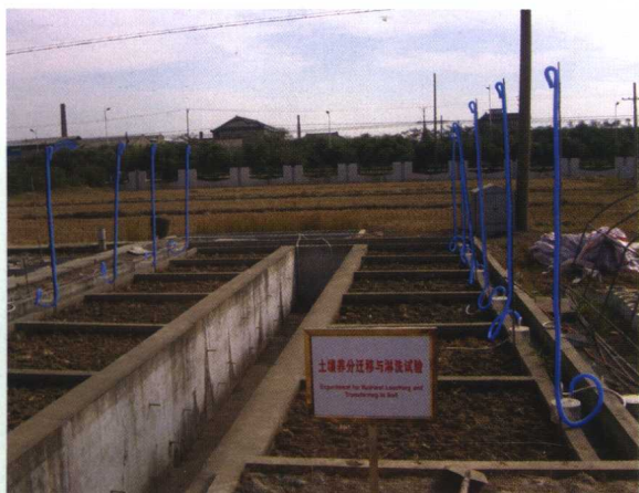
常熟农业生态站（江苏）的水稻土氮素淋溶损失试验 Lysimeter experiment on N leaching from paddy soils, Changshu Experiment Station, Jiangsu Province
