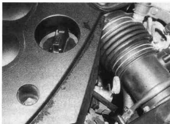
Fig. 2- 4 Notice that the engine oil fill is very close to the dipstick on this 3.5 L V6 in the Infiniti G35. Near the oil fill there is a label that warns against pulling out the dipstick ("oil level gauge") while adding oil.
