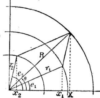
$$R^2 = r_1^2 + r_2^2 + 2r_1 r_2 \cos(e_1 - e_2),$$
