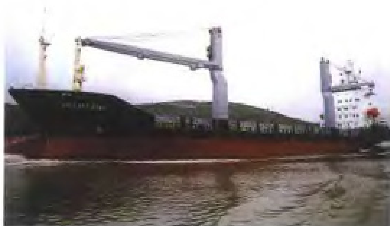
7800DWT级多用途集装箱货轮
