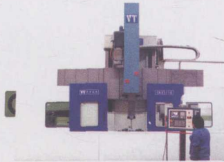
CKX51 系列单柱立式车铣加工中心 CKX51 SERIES SINGLE COLUMN VERTICAL TURNING & MILLING MACHINE
