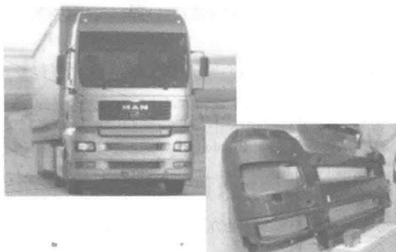
MAN TGA SMC truck bumper:34kg
