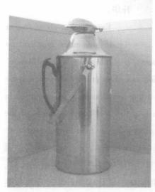
with inner surfaces silver-coated and with a vacuum space in between. The bottle is plugged by a cork. The hot water filled in the bottle can be kept warm for a long time because the glass walls and the cork stopper conduct very little heat. The vacuum space in between the glass walls prevents the heat circulation. In addition, the silver-coated inner surfaces of the glass walls reflect back the heat ra-
