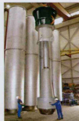
SEZ/PHZ 立式混流泵 Tubular Casing Pump
