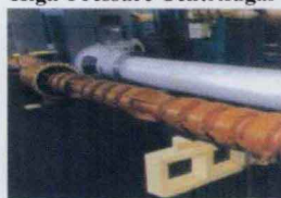
NLT 凝结水泵 Condensate Extract Pump
