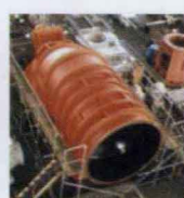
全调节斜式轴流泵 Lean Axial Flow Pump With Blade Pitch Adjustment
