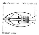
The burning of the fuel heats the air, which is forced out through the exhaust pipe 14 and provides the forward thrust. It is the smoke from the exhaust pipe which can be seen behind a jet plane in the sky. A jet plane can reach much higher speeds than a normal plane. The world's fastest jet plane has reached a speed of 2,200 miles per hour and a height of nearly 100,000 feet.
