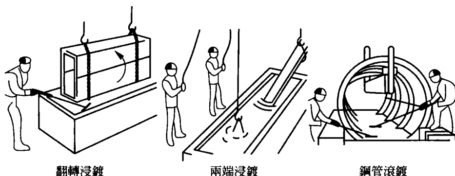
圖 1.1 大型鋼結構件在熔槽鍍鋅的過程("Galvanizing Manual", Zinc and Lead Asian Service, Melbourne, Austrian.)
