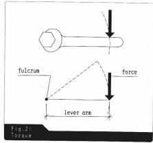
Moments, torque Forces can also work in a circle around a point. They are then called torque or moments, and are defined by their size multiplied by the distance from the fulcrum (lever arm).
