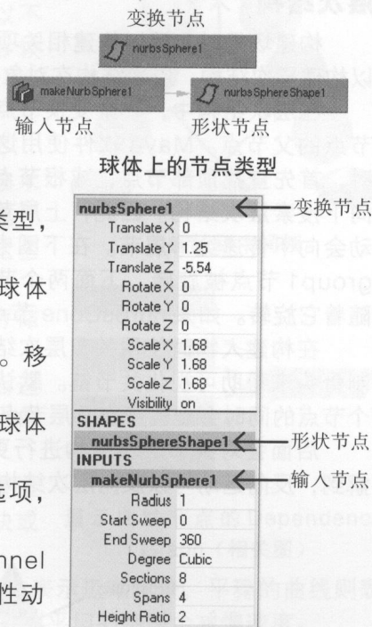
Channel Box (通道框)
