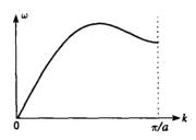
Fig. 1.2 Typical dispersion relation for phonons along a chain.
