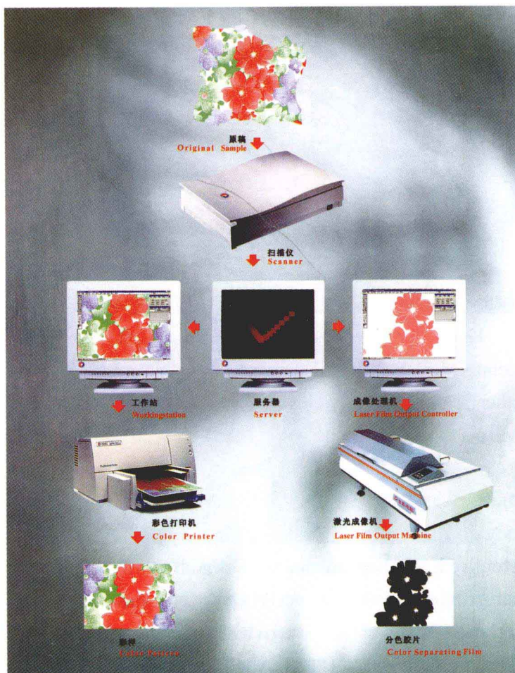
Figure 4. Flow chart of configuration and technical process for printing CAD
