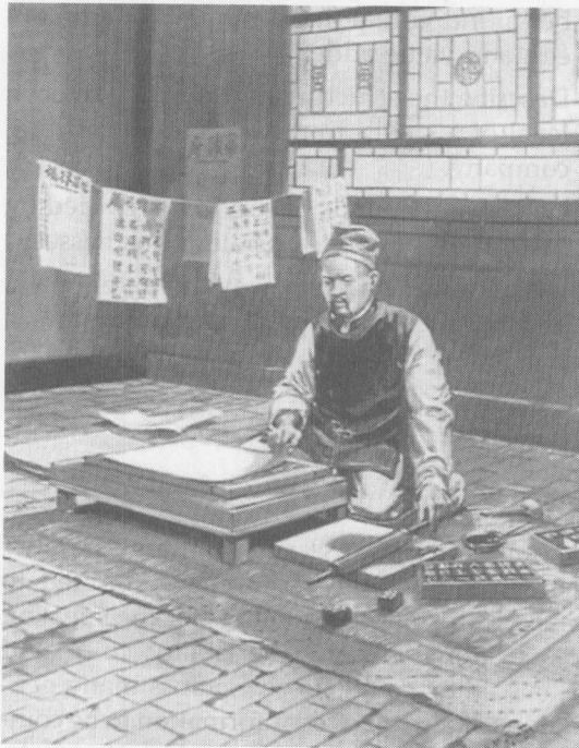
An early Chinese press. The press was a low, flat table solid enough to hold the form in place. The Bettman Archives.
