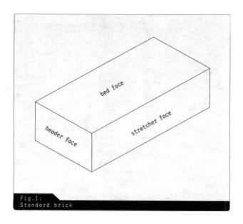
their character to most masonry façades and are firmly linked with our idea of masonry. But there are a whole variety of different shapes and sizes: flat Roman bricks, large manufactured blocks or octagonal moulded bricks. And the brick forms the basis for the whole set of craft rules of erecting a masonry building, even today. These rules govern the size of rooms and buildings, apertures and built-in features, and they structure façades.
