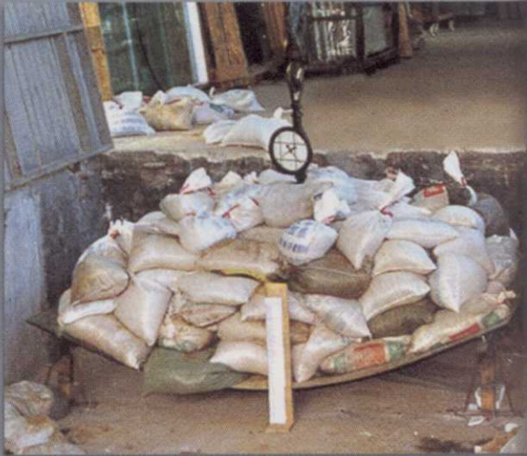
● 3000mmX2000mm 点支式玻璃支撑挠度实验情形
