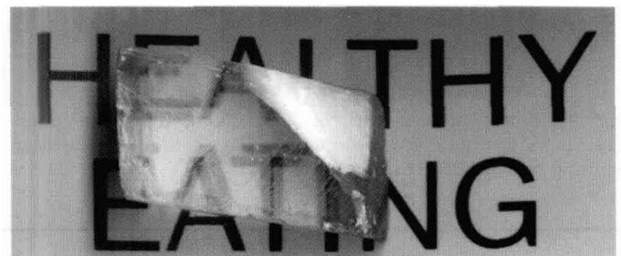
Fig. 27 A calcite crystal laid upon a paper with some letters showing the double refraction.
