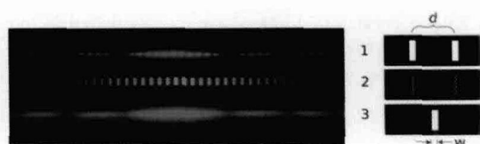
Fig. 21 1. A diffraction pattern formed by a real double slit. The width of each slit is fairly big compared to the wavelength of the light. This is a real photo. 2. This idealized pattern is not likely to occur in real life. To get it, you would need each slit to be so narrow that its width was comparable to the wavelength of the light, but that's not usually possible. This is not a real photo. 3. A real photo of a single-slit diffraction pattern caused by a slit whose width is the same as the widths of the slits used to make the top pattern.
