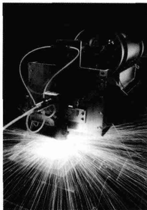
Fig. 33 A 2 kW fiber laser mounted to a robotic system cutting mild steel. Figure downloaded from the Internet.
