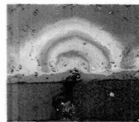
Fig. 13 A pattern of coloured light formed by interference between white light being reflected from the surface of a thin film of diesel fuel on the surface of water, and the diesel-water interface; photo taken by Dr. Guinnog.
