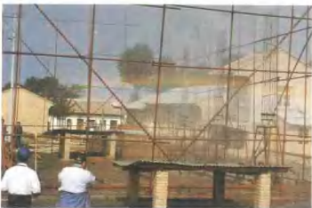
西峰水土保持科学试验站的人工降雨径流试验场 Experiment plot fed by artificial rain in the Xifeng Water and Soil Conservation Experiment Station
