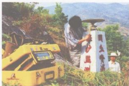
秭归卡子湾滑坡GPS监测
