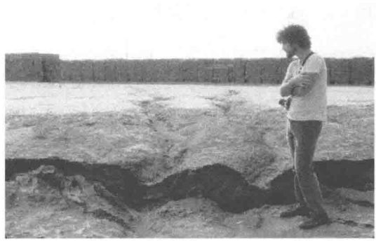
Fig 1.1 Ground rupture along the northern trace of the Imperial Fault in southern California after the October 15, 1979, magnitude 6.5 earthquake. View is to the southwest. The strike and dip components of slip are identified based on the offsets of the small stream channels. The relative motion is right-lateral strike slip (~5 cm) and dip slip (~20 cm) down to the northeast. See website for color image. Photograph by D. D. Pollard.
