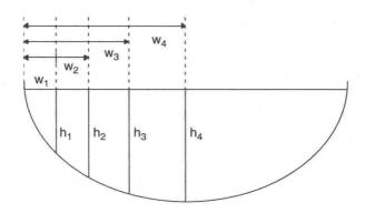
$Q = \text{Sum (mean depth} \times \text{width} \times \text{mean velocity)}$
